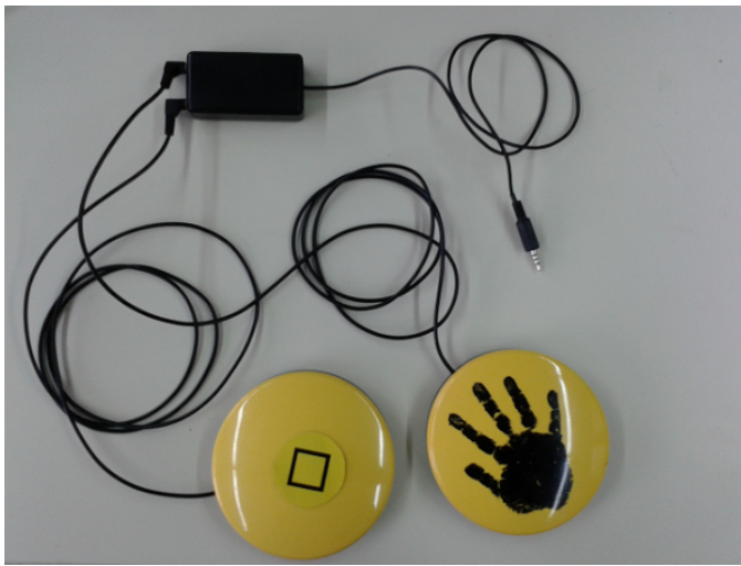
Fig. 5. The headset adapter connected to two switch sensors.
