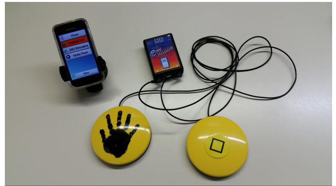
Fig. 2. A prototype of the system: smartphone, gateway, and two switches (headset adapter not shown).
